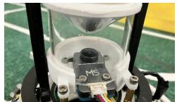
Switching the camera from OpenMV to UnitV has improved the code extensibility of the system. Coupled with tailored firmware, **the change has improved.** With the introduction of the new camera system, offensive units have an easier time shooting at the goal, and defensive units find it easier to maintain their position, **enhancing the quality of control.**
