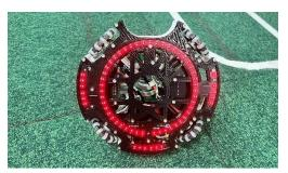
By arranging the luminance sensors in a large circular pattern, white lines **can be detected accurately and over a wide area.** Additionally, by installing luminance sensors as subsensors on the outside circle, the detection speed of white lines is improved. Furthermore, by adopting the STM32F446RE as a subCPU, similar to the ball sensors, **highspeed data processing is achieved.**
