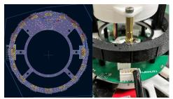
This platform is equipped with 16 high-precision ball sensors, capable of accurately detecting balls from all 360 degrees. Additionally, by adopting the STM32F446RE as a sub-CPU, **it achieves high-speed data processing.** The design of the sensor cover narrows the window opening while **ensuring that balls from the intended direction are reliably captured.**
