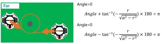
Flanking is performed using the tangent of a circle. If the distance is far, create a circle of any size centered on the ball and proceed towards its tangent. If the distance is close, flank at a 90-degree angle. Once in front of the ball, move forward towards the goal. This method improves code readability and **allows for efficient and accurate shortest distance flanking by simply changing the radius of the circle for adjustments.**
