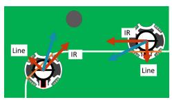
By integrating the calculations of the IR sensor vetor with the Line sensor vector, stacking actions were eliminated, **allowing for rapid movement towards the ball.** The Line sensor has been improved to accurately capture the angle at which the machine intersects with the line. This enhancement allows for clean line tracing at the goal ends, approaching the ball smoothly, and stopping precisely at the edges, making **it easier to block shots**.
