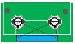
We use cameras to constantly recognize our goal, so we can keep track of where we are. **This allows us to precisely calculate Current coordinates on the field.** As a result, we no longer get stuck on the edge of the court and can't get back. Furthermore, if we are pushed out of the goal area by an opponent or our own machine, we can return to the goal and **efficiently return to our original position.** This stabilizes our vehicle.
