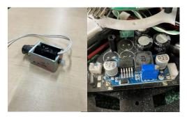
The ability to score goals has improved. By changing the resistor connected to the capacitor in the boost circuit that supplies power to the solenoid to a cement resistor,
