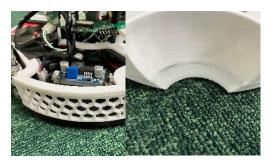
In pursuit of making the body lighter, a honeycomb structure was adopted for the walls, and the top plate was designed to be as minimal as necessary. Furthermore, by angling the hold area, the previous issue of balls bouncing out of the hold area has been resolved. This improvement ensures reliable ball holding, which in turn has increased the success rate of shots on goal.
