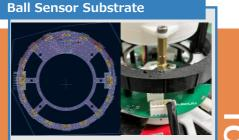
This platform is equipped with 16 high precision ball sensors, capable of accurately detecting balls from all 360 degrees Additionally, by adopting the STM32F446RE as a sub-CPU, it achieve ph-speed data processing. The design of the sensor cover narrows the window opening while ensuring that balls from the intended direction are reliabl aptured.
